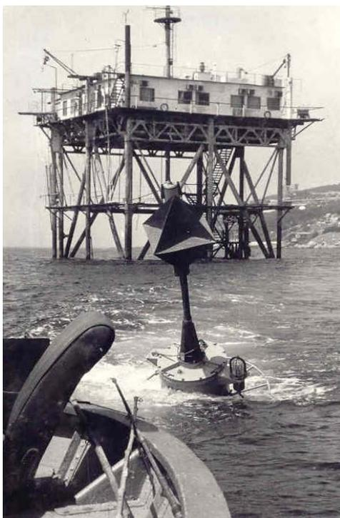
**Fig. 2.** MHI-9301 drifter with RNS “Omega” receiver and satellite transmission system SSPI-IK equipment during the tests in the area of oceanographic platform in Katsiveli
