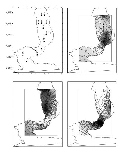
**Fig. 1.** Spatial distribution of the stations in the Balaklava Bay in 2005 where the following samples of the bottom sediment surface layer (0 - 5 cm) were taken: bottom sediment (*a*) and the granulometric composition fractions, i.e. sand (*b*), silt (*c*) and gravel (*d*)
