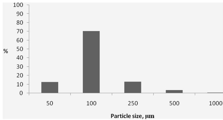
**Fig. 5.** Diagram of the percentage of the sediment fractions in accordance with the results obtained by the standard sieve method
