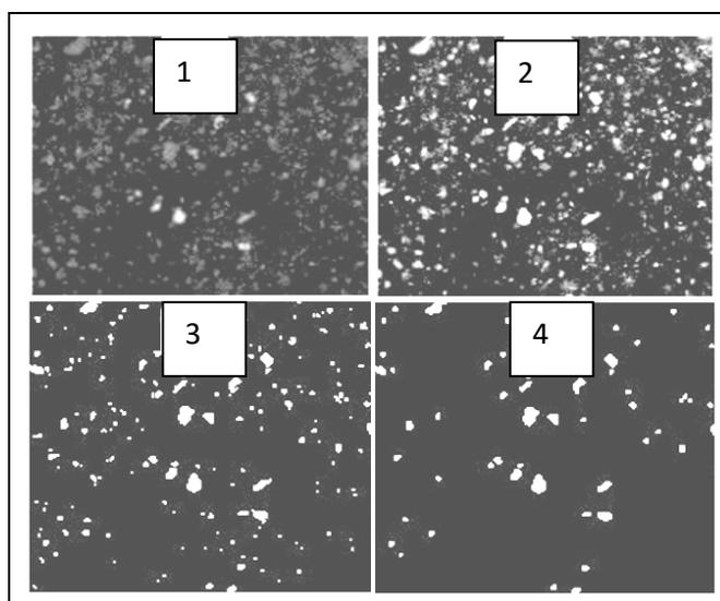
**Fig. 2.** Stages of processing of the images obtained: 1 – original image; 2 – image pre-processing result; 3, 4 – image after segmentation and filtration
