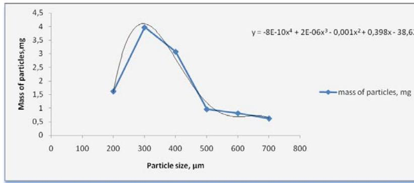
Fig. 4. Mass distribution of the particles for each fraction
