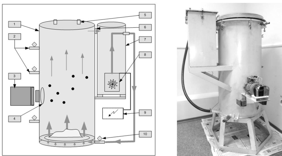
**Fig. 1.** A construction diagram and photo of the test stand: 1 – steel tank; 2 – valves for sampling; 3 – photorecorder; 4 – porthole; 5 – sealed cover; 6 – a connecting branch for water return to the tank; 7 – pumping container; 8 – pump
