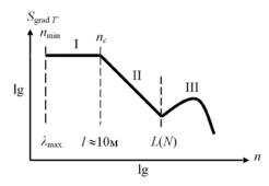
Fig. 1. Scheme of vertical spectrum of temperature fluctuation gradients in the main thermocline proposed by M. Gregg [12]
