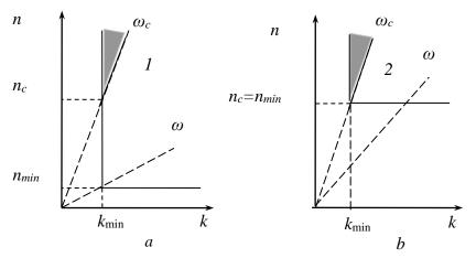
**Fig. 4.** The areas of quasi-inertial internal wave energy loss (darkened) according to model [8] for "weakly" stratified (*1* in fragment *a*) and "strongly" stratified (*2* in fragment *b*) layers
