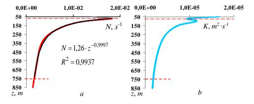
**Fig. 5.** Average over 70 years N(z) buoyancy frequency distribution over the depth in the Black Sea (exponential approximation of initial relation) – a; K(z) model relation – b. Red dashed lines denote the depth of N maximum location and the maximum depth down to which the model is valid
