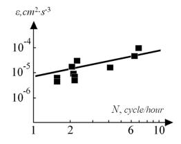
**Fig. 3.** Ensemble-averaged values of kinetic energy  $\varepsilon$  dissipation rate depending on *N* from the paper [6] (squares). Straight line corresponds to expression (5)
