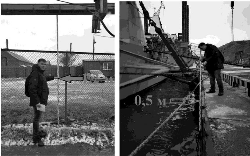
**Fig. 3.** Measurement of the runup height resulted from the storm surge in the port of Korsakov
