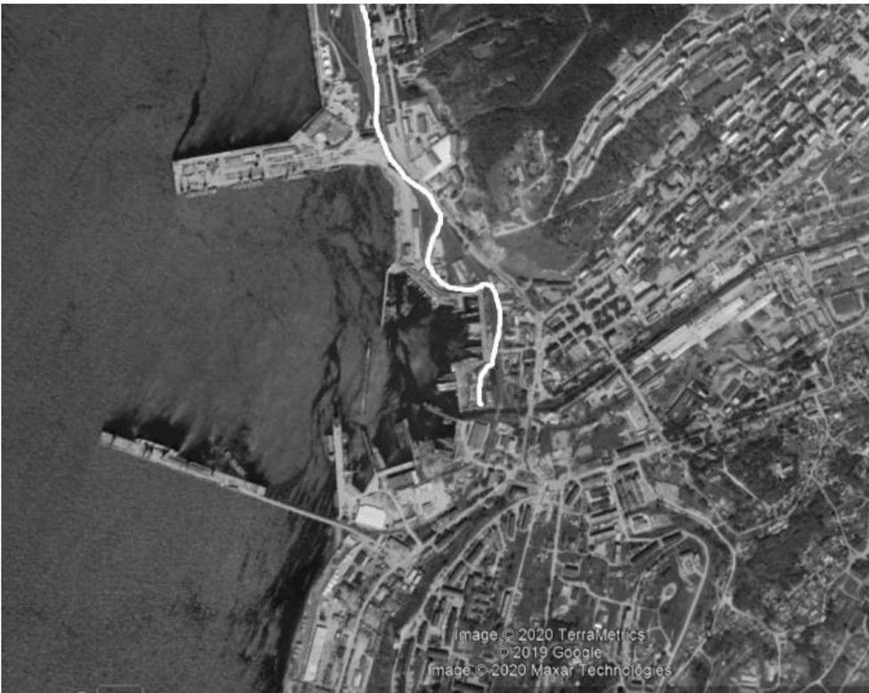
**Fig. 2.** Zone flooded due to the storm surge on 15.11.2019 (white line marks the GPS-track of the runup boundary)
