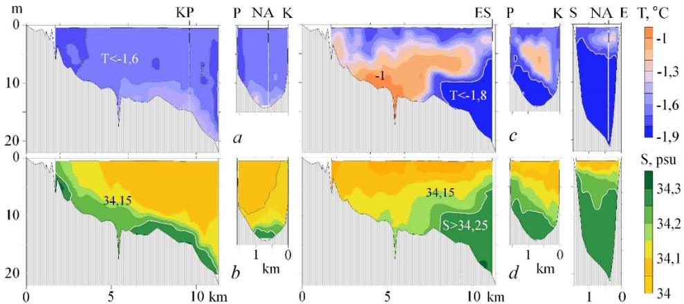
**Fig. 5.** Temperature (*a, c*) and salinity (*b, d*) measured by the *ASTD102* probe on the axial section *NA* and on the cross-sections *vil. Kanal – vil. Podnozh'e (KP)* and *Elena Island – Staritsky Cape (ES)* on February, 1 (*a, b*) and February, 23 (*c, d*), 2017
