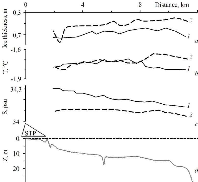
**Fig. 6.** Ice thickness (*a*), temperature (*b*) and salinity (*c*) of the water column; bottom topography (*d*) on the axial section NA in the Novik Bay based on the observation data of February 23, 2013 (1) and February 24, 2016 (2). Triangle with inscription “STP” denotes location of the sewage treatment plants of the FEPU campus
