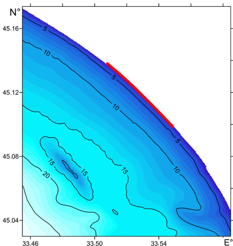
**Fig. 7.** Model bottom topography in the region of the Sakscoe Lake bay-bar. Red line shows the design area
