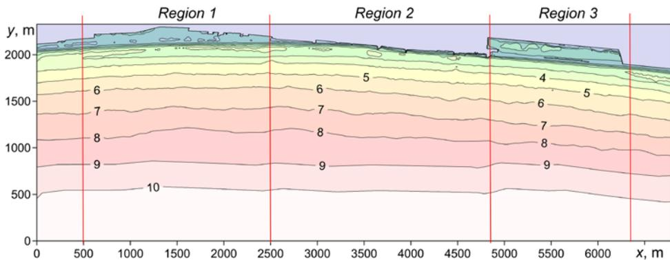
**Fig. 8.** Bottom and land relief (m) of the coastal zone for modeling the wave run-up on the coast and the beach profile deformations
