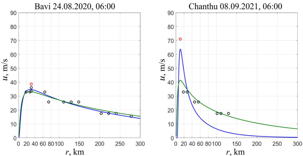
**Fig. 2.** Examples of approximating the data on wind speed (black circles) in the TC *Bavi* and *Chanthu* by the Holland function (1) (blue line denotes the TC near zone, green one – the TC periphery; red circles are the radius and the maximum wind speed based on the Best Track Data)
